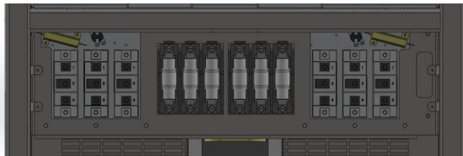
FIGURE 12 POWER MODULE FUSES
