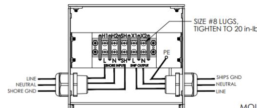
TYPICAL ELECTRICAL WIRING
